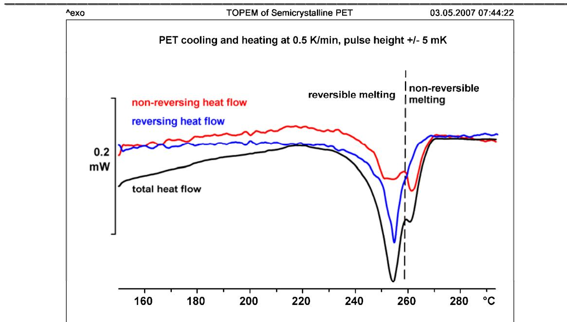
**Figure 6.** The melting behavior of PET that had been previously cooled at 0.5 K/min shows two different melting processes.
