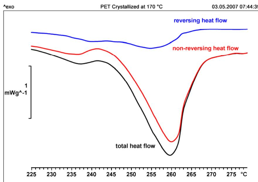
**Figure 5.** Heat flow curves in the melting region of PET that had been crystallized for 10 min at 170 °C. The underlying heating rate was 0.3 K/min.
