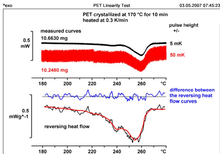
**Figure 2. Test of the linearity condition using PET that had been crystallized at 170 °C. Above: measurement curves. Below: reversing heat flow and the difference between the two curves (blue).**
