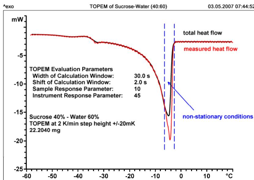
Figure 3. TOPEM® measurement in the melting region of a sucrose–water mixture.
