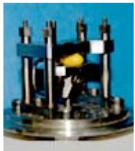
New clamps are now available for the DMA 8000. These clamps allow for the analysis of tablets for mechanical properties.
