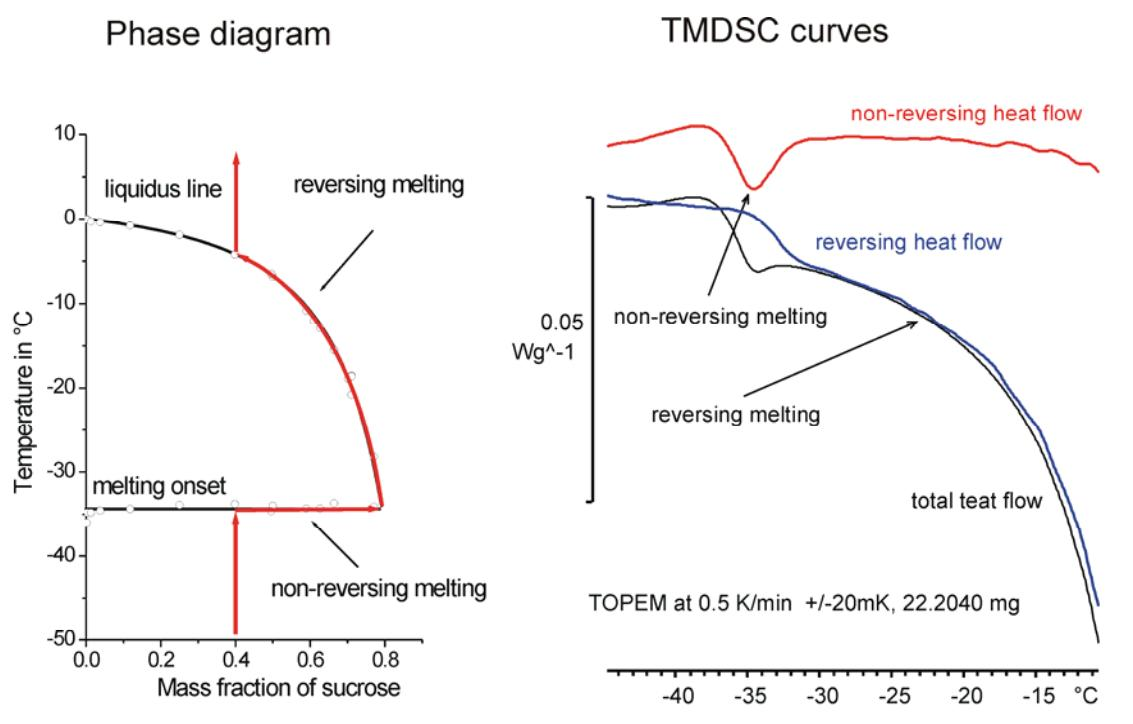
**Figure 4.** Left: Simplified phase diagram of a sucrose and water mixture. The path taken by the measurement is marked by red arrows. Right: Curves obtained from a TOPEM® measurement.
