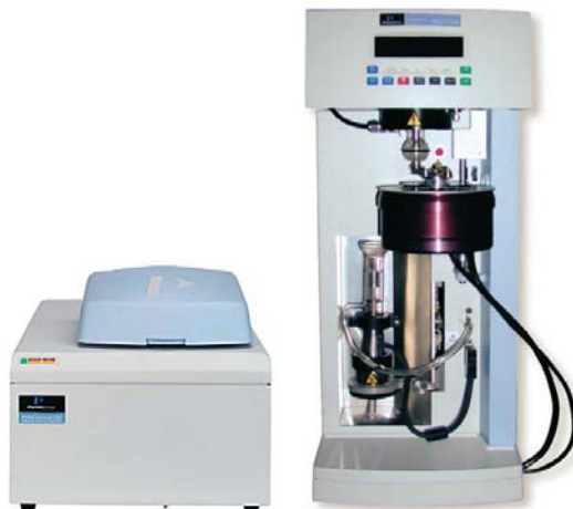
Figure 1. The Diamond DSC (left) and Pyris 1 TGA (right) represent the state of the art in modern thermal analysis.
