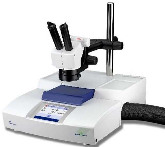
Fig. 1. The Flash DSC1 with microscope and connection to the intracooler
